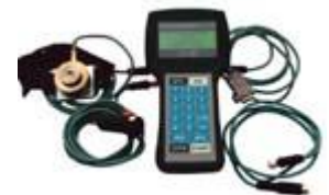
CL 170 Set with force sensor on brake pedal
