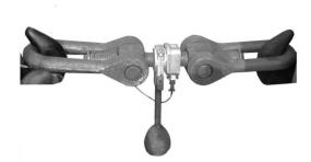
Strain gauge force sensor CL 15K is assigned for measurement of locomotive tractive forces. The sensor was build as a reconstruction of standard railway screw coupling. A fragment of screw coupling is an elastic element of sensor working tensile. The elastic element is bonded with strain gauges building a balanced and thermal compensated bridge. The sensor can cooperate with measurement instruments from other producers.
