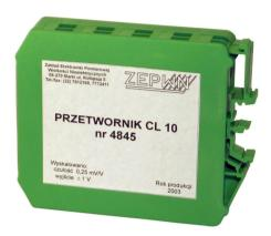
DC amplifier CL 10 is assigned for use with a single strain gage sensor with  $120 \div 1200~\Omega$  full bridge. The amplifier can be used to gain signal from strain gage force sensor, weight load cells and pressure sensors. It is especially suitable for applications in difficult climatic and mechanical environment. This amplifier is assigned for industrial use and other environments demanding high protection against dust, vibrations and humidity.
