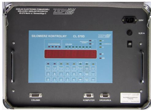
The Control force meter CL 570D is a force standard with accuracy class 0,5 or 1. CL 570D is assigned for calibration of operational force meters and testing machines. The device is compatible to any force sensor. A program used in the device allows to do cyclic force measurements and its presentation on the digital display. Program procedures analyze measured forces and signalize overflow of two limiting values for every sensor.
